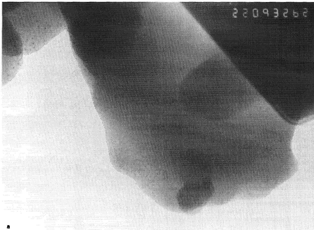
FIG. 1. (a) Micrographs of 0.5 wt% Pt-silicalite (0.7 nm = 1.5 nm). (b) Micrographs of 0.5 wt% Pt-Na ZSM-5 (0.7 nm = 3 nm). (c) Micrographs of 4 wt% Pt-silicalite (0.7 nm = 3 nm).
